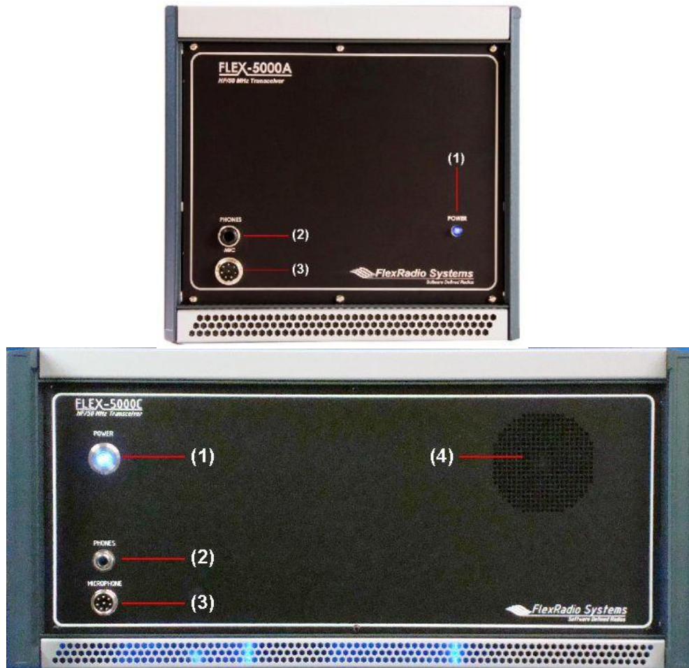
Figure 2: FLEX-5000A (top) and FLEX-5000C (bottom) Front Panel
