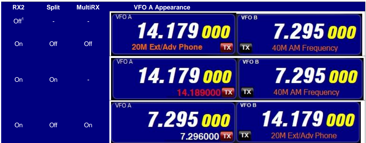
Figure 47: VFO A and VFO B (with RX2 present and ON)
