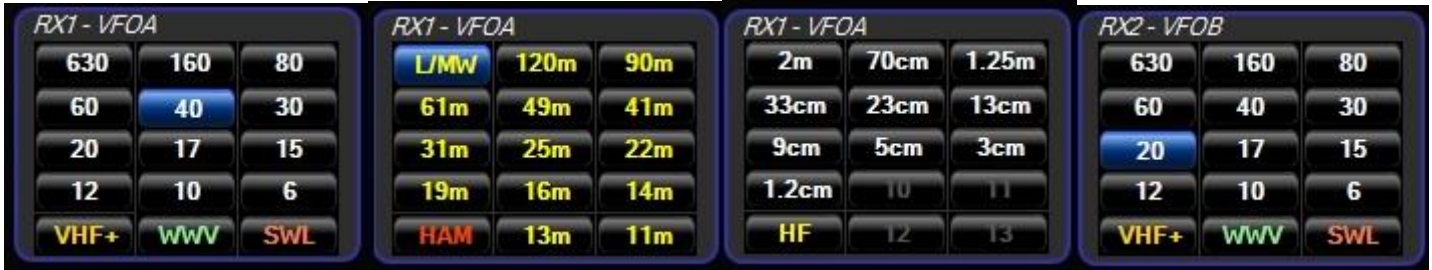
Figure 51: Primary (left) and RX2 (right) Band Selection
