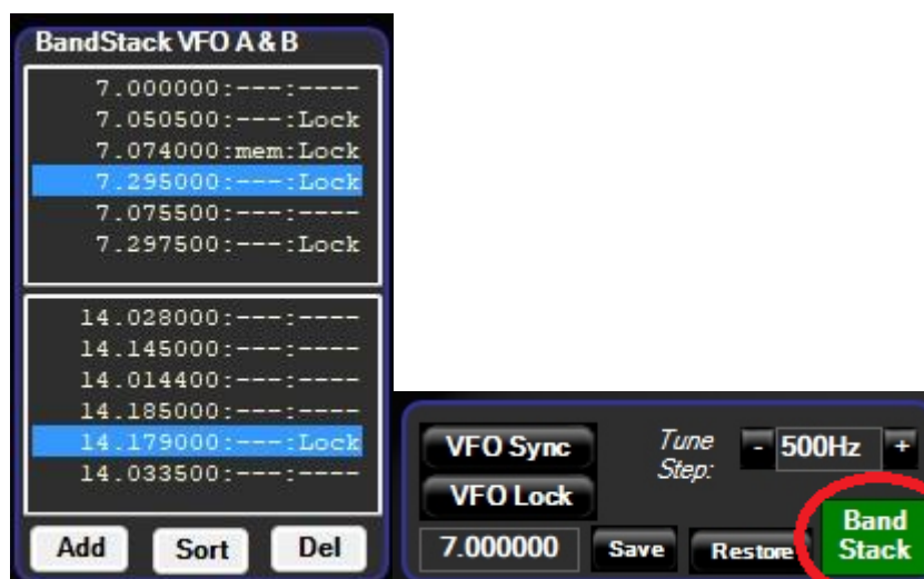
Figure 51a: Click on BandStack button (turns Green) to enable BandStack window
